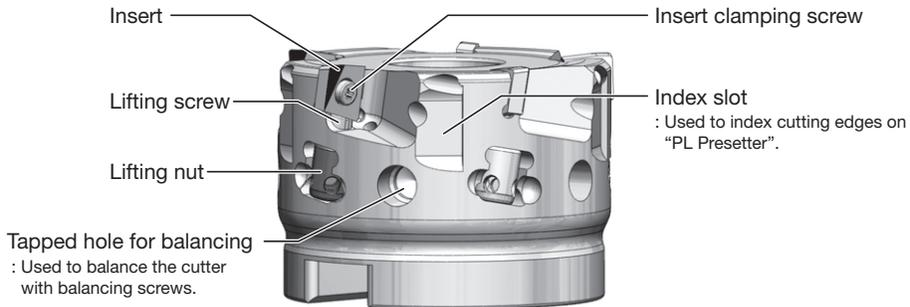
When a cutter is used at a higher rotational speed than  $12,000\text{min}^{-1}$ , request **BIG** to balance the cutter attached to a toolholder.
