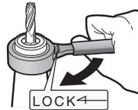
※To ease the application of the MEGA WRENCH to the chuck it is suggested to rotate in the reverse direction while sliding into position.
