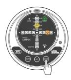
②Adjust the level in order to turn on the LED (blue) of the central position. When the inclination of one of the axes is adjusted within 0.01, the LED (blue) turns on and the buzzer emits a sound [Beep, beep]. When the inclination of both axes is within 0.01, the LED (blue) turns on and the buzzer emits a sound [Beep-beep-beep].
